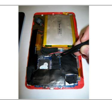
Remove the black adhesive strips from the wires using the tweezers, and set the strips aside.
