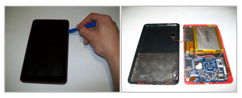
Use the plastic opening tools to pry the screen from the back of the device.
