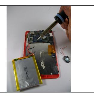
Using the soldering iron, apply heat to the end of the wires until they are free from the motherboard.
