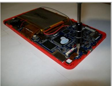
Unscrew the motherboard using a J0 Phillips head screwdriver.
