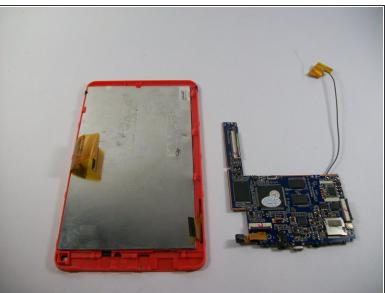
Now that the battery and speaker are removed, the black clips are undone, and the motherboard is unscrewed, remove the motherboard.
