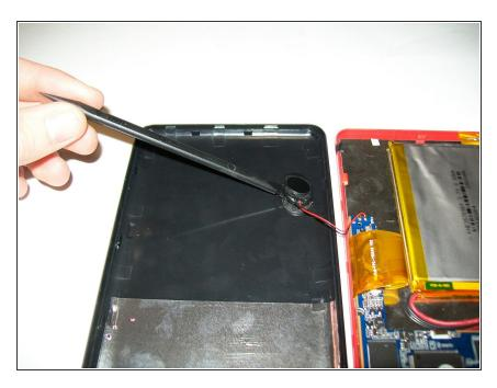
Use the spudger to remove the speaker from the back casing of the device.
