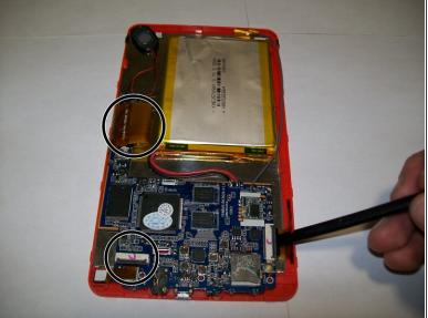
• Use the spudger to release three (3) black clips connecting the components to the motherboard.
