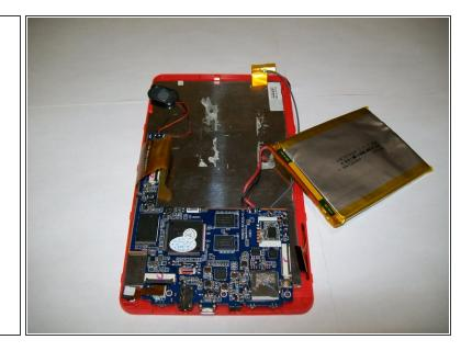
Use the metal spatula to remove the battery from the back of the screen.
