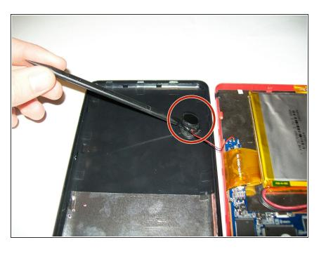
Use Spudger to remove speaker from back casing of the device.
