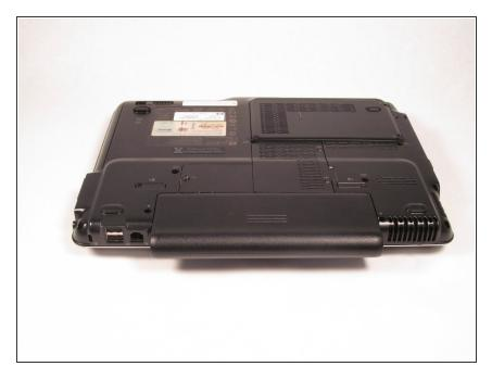
Completely power down and unplug the device. Lay device flat on a soft surface upside down.
