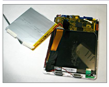
The battery is now disconnected from the tablet and can replaced. Reinstallation of the new battery and tablet assembly can be completed by following the same steps in reverse.
