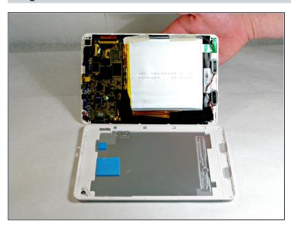
You should now be able to separate the two halves of the tablet. Set the back cover aside since you will not be needing it until reassembly.
