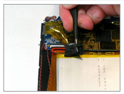
Use <u>tweezers</u> to slowly lift the black adhesive strip off of the battery's soldering points.
