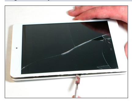
Starting near the middle edge of the Trio Stealth-G4X tablet, gently work the pry tool in between the seams of one side of the tablet.
