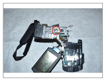
The speaker is now removed, and the speaker port is open. Replace the new speaker with the damaged one, and replace the one 3mm screw To reassemble your device, follow these instructions in reverse order.
