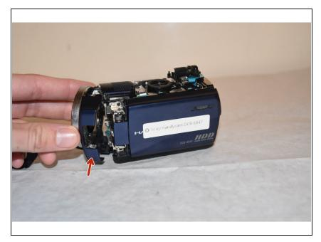
Carefully remove the lens covering from the camera in order to access the internal components
