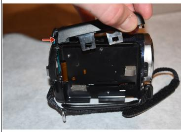
Using the spudger, remove the top housing where the hard drive was located.
