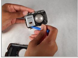
Once the two 2mm screws and the 3 mm screw have been removed, use the smallest plastic opening tool and pull up on the sides to reveal the inside of the camera.
