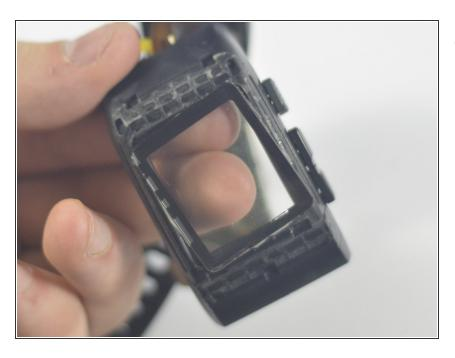
Push the panel out from the back of the screen, using your fingers.
