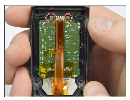
Two size #000 2.5 mm long screws will appear at the top of the main board. Unscrew them using a size 000 Phillips head screwdriver.
