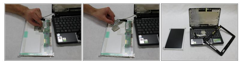
Gently pull the tab that is connecting the laptop to the screen, to fully disconnect the screen from the laptop.
