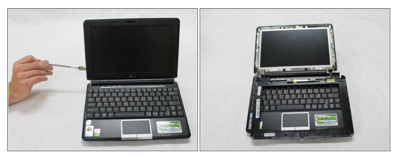
• Use the metal spudger to pry off the outside frame of the screen.
