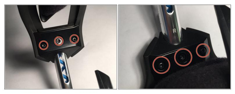
Remove the six screws—three from each side of the headband
