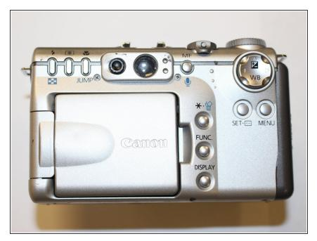
Start by removing all of the screws around the camera: from the front, back, sides, and bottom.
