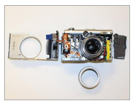
Next remove the front and right side panels (the left side is attached to the front panel).
