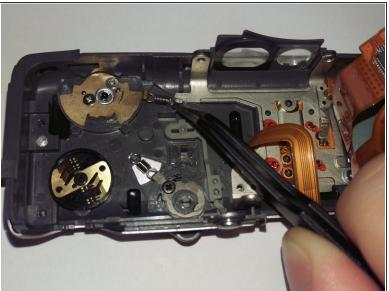
Replace the zoom control spring with a comparable spring, attaching the loop ends to the same metal pegs to which the previous spring was attached (on the panel and zoom control.)
