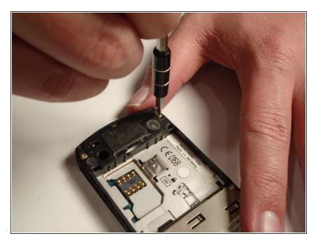
Use a screwdriver with a T6 Torx screwdriver head to remove both screws (1/8") from the speaker housing. Turn the screw counterclockwise (left).
