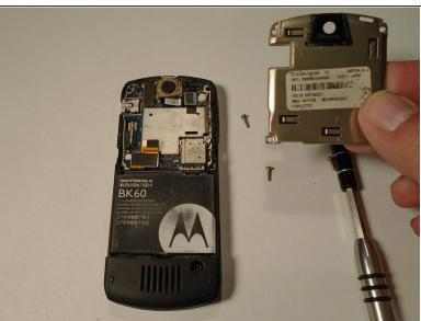
Once you have removed all of the screws, lift the transceiver PC board shield up to remove it.
