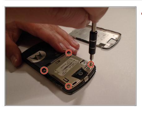
Remove the four housing screws (1/8") from each corner of the transceiver PC board shield. Use a screwdriver with a T6 Torx screwdriver head to turn the screws counter-clockwise (left).
