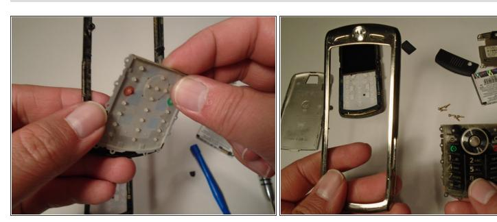
Lift the keypad up from the front plate to remove.
