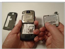
To remove the battery, pull the battery up from the bottom center.
