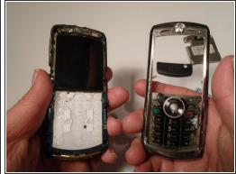
Using the grooves around the edge of the phone, gently pull the front plate away from the phone until it is fully removed from the device.
