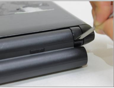
Wedge the nylon or metal spudger inside the gap and pry open the two plastic parts.
