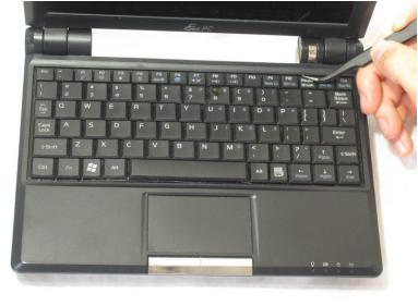
• Flip the laptop back over and unlock the three keyboard tabs at the top of the keyboard by pushing down on the silver tabs with tweezers.
