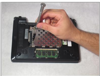
Remove the screw under the hard drive using the Phillips J0 Screwdriver.
