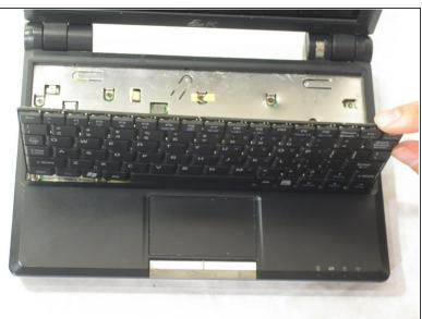
Use the plastic opening tool to lift up the keyboard.
