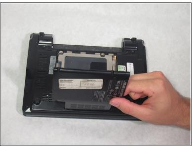
Using a plastic opening tool, take off the hard drive cover by lifting it up.
