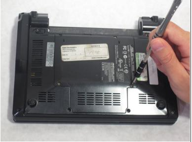
Remove the four 4.76 mm screws using the Phillips J0 Screwdriver.
