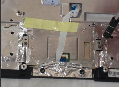
• Remove the two 4.76 mm screws using the Philips JO screwdriver.
