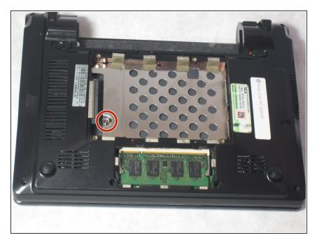
Remove the 4.76 mm screw under the hard drive using the Phillips J0 screwdriver.
