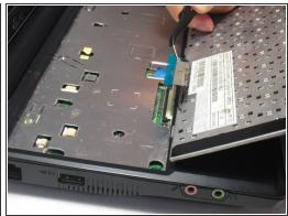
Using a pair of tweezers, disconnect the cable at the bottom of the keyboard by flipping the two black lock switches up on both sides of the cable.
