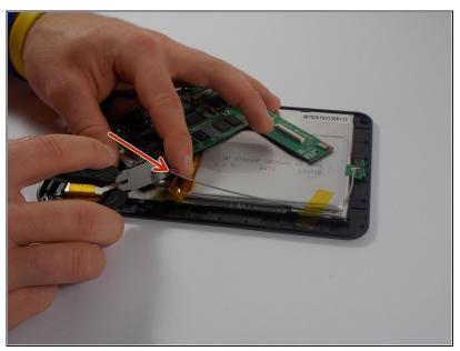
⚠ Using wire cutters, cut only the **gray** wire.
