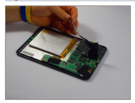
Remove any static tape covering the motherboard.
