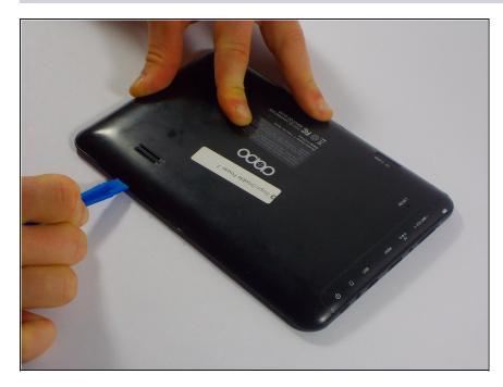
• Carefully, wedge the plastic opening tool in-between the seam that separates both halves of the tablet.
