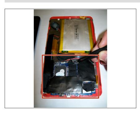
Use tweezers to remove the black adhesive strips from the wires. Set aside
