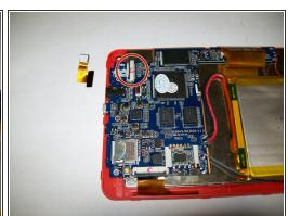
• Use a spudger to undo the black clip connecting the camera wires to the motherboard.
