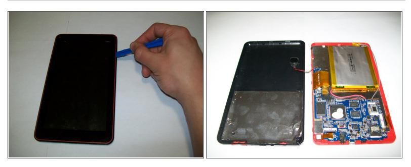
Use the plastic opening tools to pry open the back case of the device.
