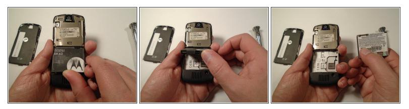
• To remove the battery, pull the battery up from the bottom center.
