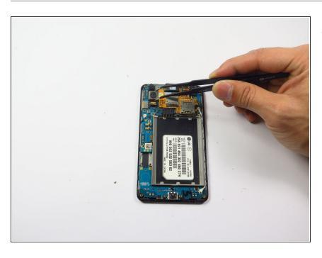
Use a pair of tweezers to disconnect and remove the rear facing camera.
