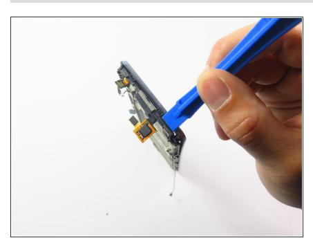
Use the plastic opening tool to remove front glass cover carefully.
