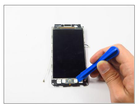
Use the plastic opening tool to carefully remove the home button board. It is attached with doublesided tape.
