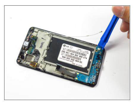
Use the plastic opening tool to remove the charging port unit.
