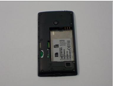
Insert the spudger into the space between the batter and the battery holder to remove the battery.
