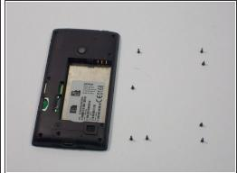
Unscrew the 8 screws with a Torx screw driver (T4). After all screws are unscrewed place them next to the phone in the order
