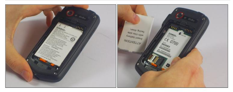
• Once the battery cover is off, there is another lock holding the battery in place. However, with this lock all you have to do is slide the lock to "Free", and pull the battery out by lifting it from the bottom side (the side with the orange lock).
