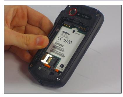
After removing the battery you will find a port that is labeled SIM directly beneath where the battery was sitting.
