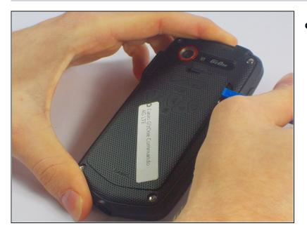
In order to get at the battery, you will have to pull the locking tab to the "Free" position. Once you do that you will have to pry the battery cover off (using a plastic opening tool or similar prying tool). Because the phone is designed to be waterproof, it is advised that you do NOT use your fingernails.
