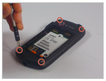
Using the same screw head, remove the back four screws from the device.
