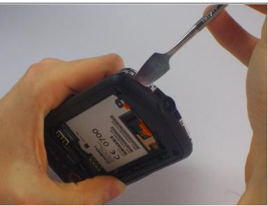
You should have taken out six screws (two from the front, four from the back). Once you do this, you will have to separate the front and back casing of the phone using a spudger or pry tool.
