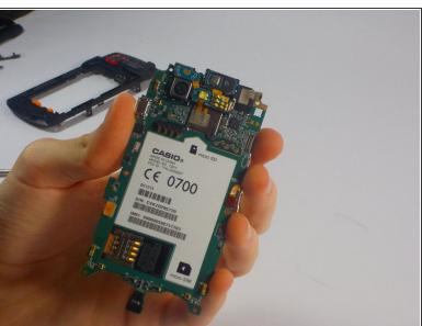
After removing the screws carefully separate the motherboard from the shell with the spudger.
