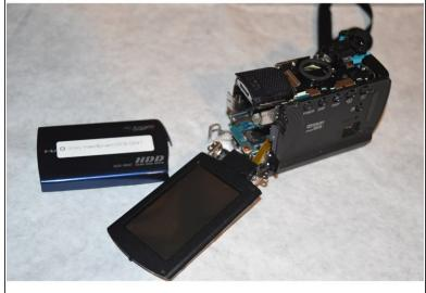
Using the plastic opening tool, separate the LCD screen from its plastic housing
