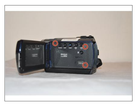
Using the Phillips #000 tool, remove the three 3mm screws from under the LCD screen
