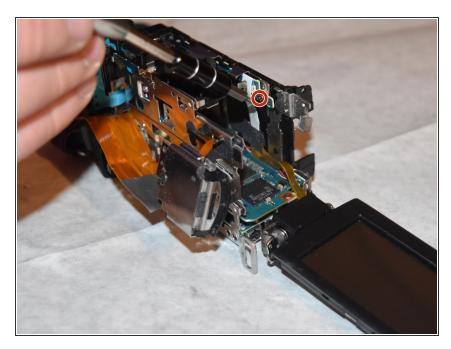
Using the Phillips #000 screwdriver, remove the single 2mm screw from under the microphone port covering
