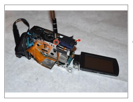
Using the Philips #000 screwdriver, remove the single 3mm screw from the top of the camera. This removal
