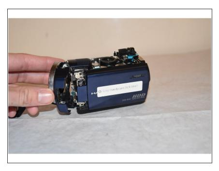
Carefully remove the lens covering from the camera in order to access the internal components
