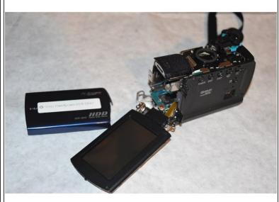
Using the plastic opening tool, carefully separate the LCD Screen from the back covering
