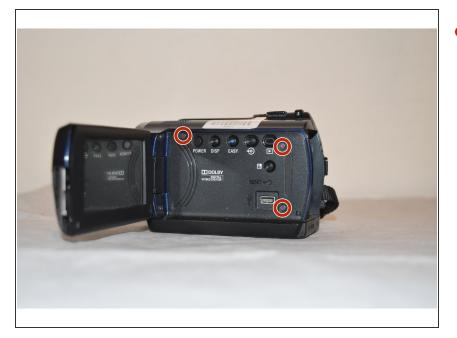
Using the Phillips #000 tool, remove the three 3mm screws from under the LCD screen
