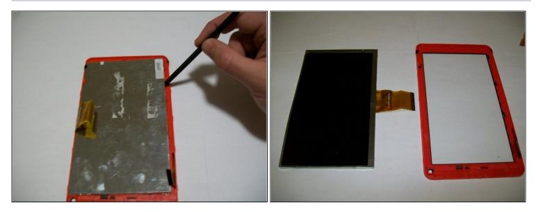
• Use the spudger to push back the clips along the side of the device and remove the screen.
