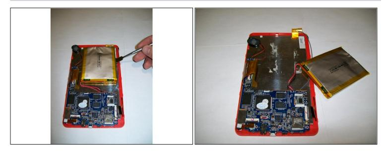
• Use a spudger to gently remove the battery from the motherboard.
