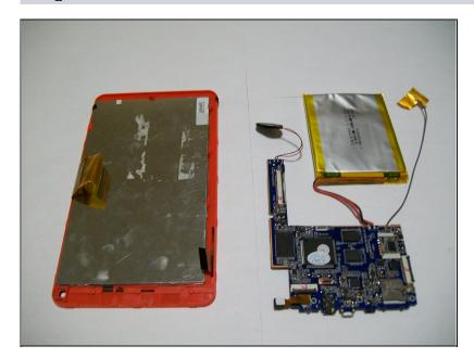
• All components will be removable from the screen after the battery, motherboard and all the black clips have been undone.
