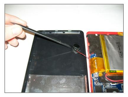
• Use the spudger tool to remove the speaker from back casing of the device.
