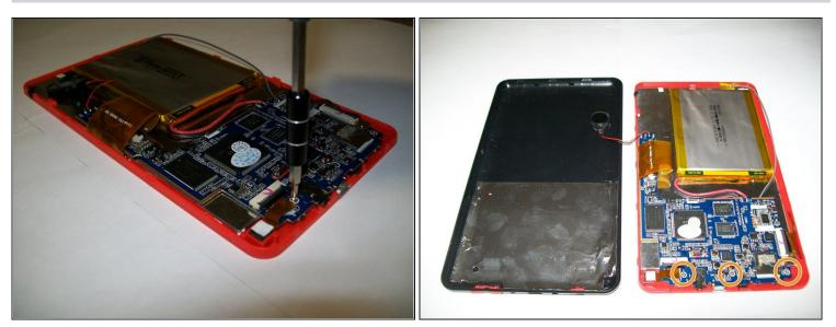
• Remove the three screws from the bottom of the motherboard.
