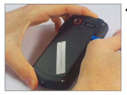
In order to get at the battery, you will have to pull the locking tab to the "Free" position. Once you do that you will have to pry the battery cover off (using a plastic opening tool or similar prying tool). Because the phone is designed to be waterproof, it is advised that you do NOT use your fingernails.
