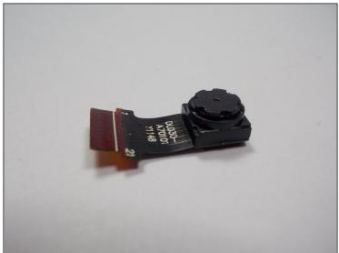
• Using <u>tweezers</u> remove the camera by the pins from the motherboard.
