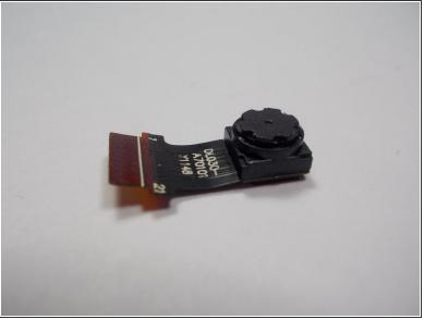
Using tweezers remove the camera by the pins from the motherboard.
