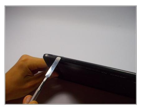
Gently go around the outside of the back plate and pry the back cover off.
