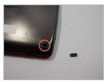
Remove all the tape and plugs to access the screws beneath.
