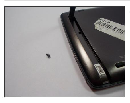
Unscrew all 5 of the .3mm t4 screws from the back plate of the device.
