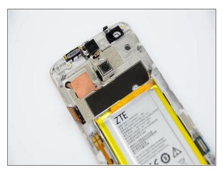
Remove the earpiece speaker, back camera and vibrator unit.
