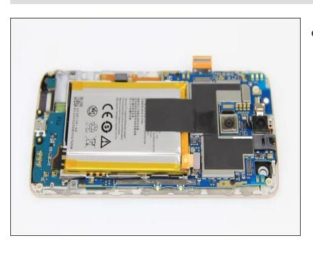
Free the RF cable and remove the screws securing the mainboard.
