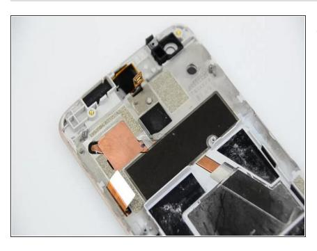
The heat pipe radiator. Remove the sub-board.
