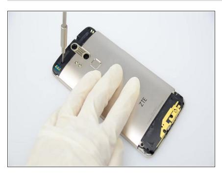
Remove the screws securing the back housing assembly.
