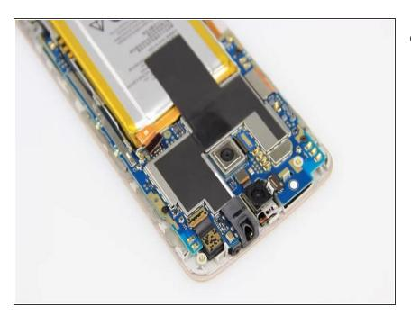
Free the front camera and disconnect the connectors.
