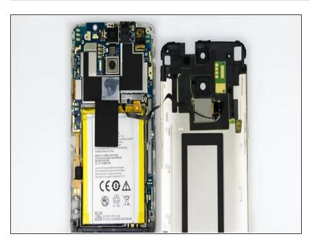
Remove the back housing assembly.
