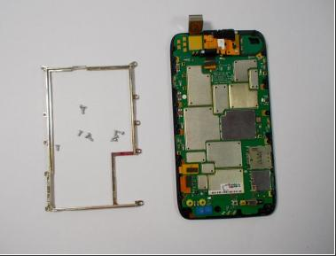
Remove the 10 Torx T5 screws, that hold the metal frame to the motherboard.
