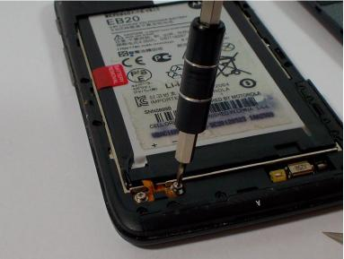
• Use the T-5 Torx bit to remove the two silver 3.3 mm screws with integrated washers.
