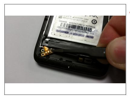
⚠ Lift the battery leads to the upward position. The ribbon cable is very thin, be gentle.
