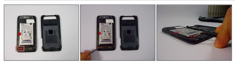
• Remove the red rubber screw cover with a pair of tweezers
