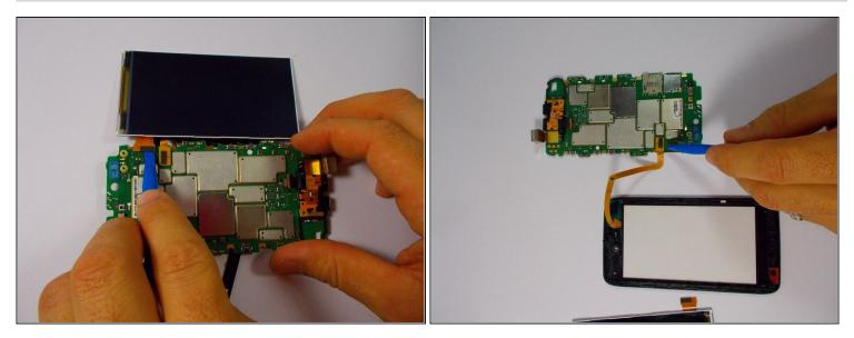
A Remove the ribbon cable connecting the LCD display to the motherboard, be mindful that the ribbon cable is very thin.
