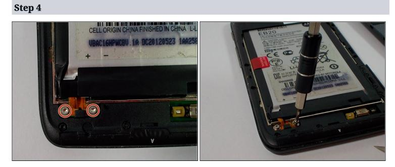
• Use the T-5 Torx bit to remove the two silver 3.3 mm screws with integrated washers.
