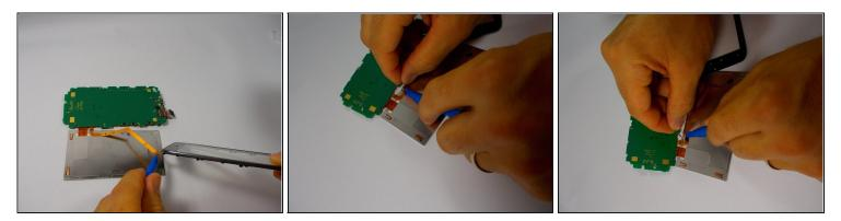
• Remove the ribbon cable from the back of the lcd using the plastic opening tool or spudger.
