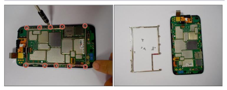
• Remove the 10 Torx T5 screws, that hold the metal frame to the motherboard.
