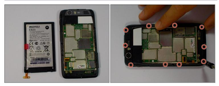
(i) The back case portion may be removed after the battery has been removed.
