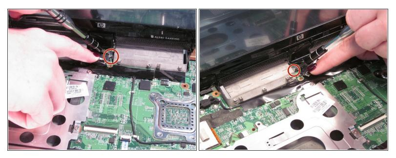
• Using the Phillips #0 screwdriver, remove both of the 5.0 mm screws on the base of the rotator.
