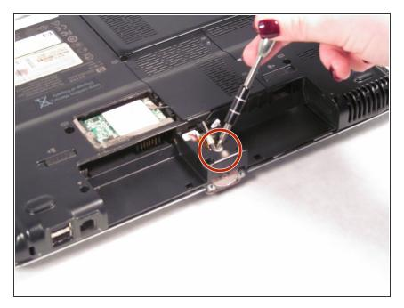
Using the Phillips #0 screwdriver, unscrew the 4.5 mm screw from the middle section in the battery compartment.
