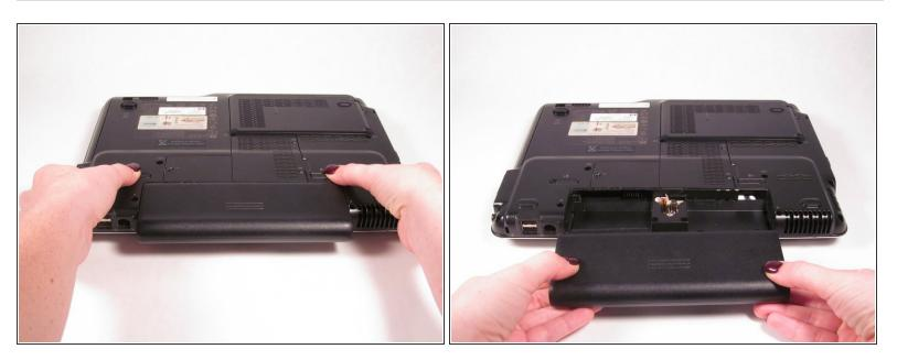
• Squeeze the latches on the battery until you hear a click. Slide out the battery.
