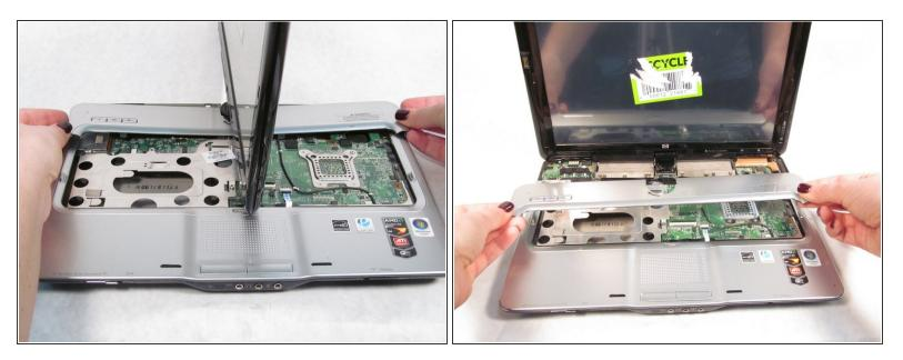
• Rotate the screen 90 degrees and remove the base under the screen.
