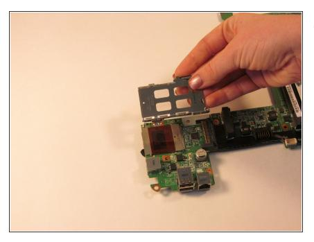
• Gently remove the bezel from the system board.
