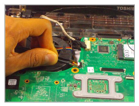
Detach the cable connecting the fan to the motherboard.
