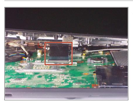
Detach the ribbon cable that connects the keyboard to the motherboard.
