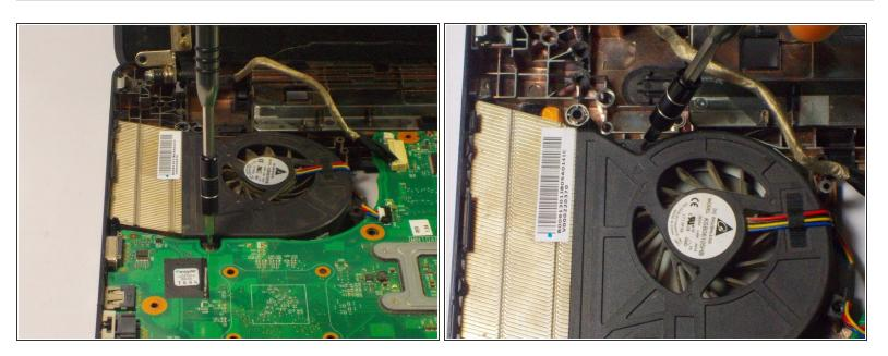
Remove the one 3.0mm and one 5.0mm Philips #0 screws holding the fan in place.
