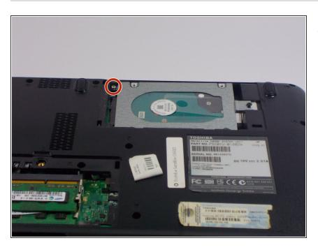
Remove the one 3.0mm Philip's #0 screw holding the hard drive in place.
