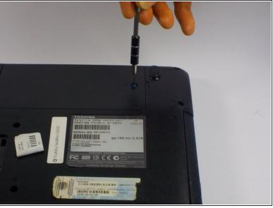
Remove the one 5.0mm Philips #0 screw that holds down the panel covering the hard drive.
