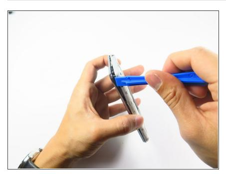
Separate the rear plastic case by inserting the opening tool between the seams on all sides.
