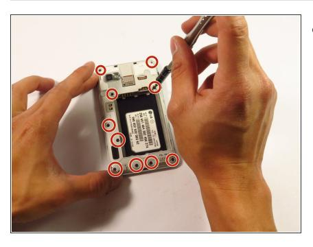
Unscrew the ten 1.0 mm screws on the back.
