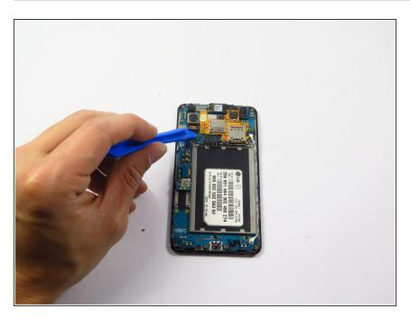
Use a plastic opening tool to detach the connector between the back camera and the motherboard.
