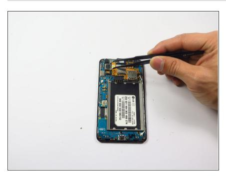
Use the tweezers to remove the camera by pinching the sides and carefully pulling up.
