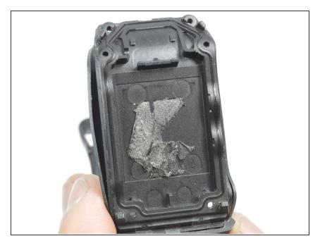
After taking the battery out, you will be left with just the band and the backpanel part of the watch.
