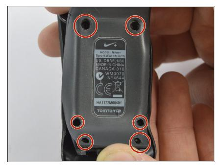
Face the watch upside down, so that the back of the watch is exposed. Unscrew the six #000 size 5 mm long screws on the back using a size 000 Phillips head screwdriver.
