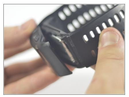
Carefully separate the watch by pulling the band away from the main board.
