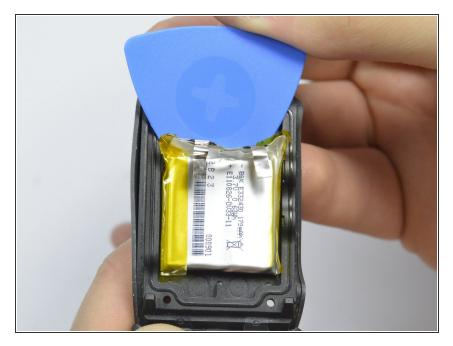
Using a guitar pick removal tool, push under the battery to pry the battery out of the watch.
