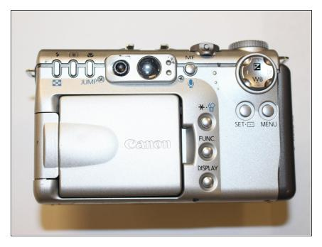
Start to remove the screws around the camera: from the front, back, sides, and bottom.
