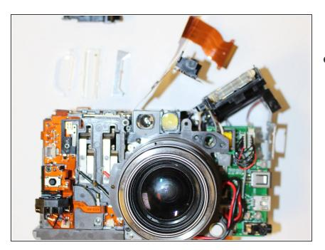
To remove the circuit ribbon (brown strip) pull it out of the plastic piece it is connected to.
