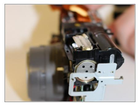
You should now be able to see how the capacitor/speaker housing slides out of the frame.
