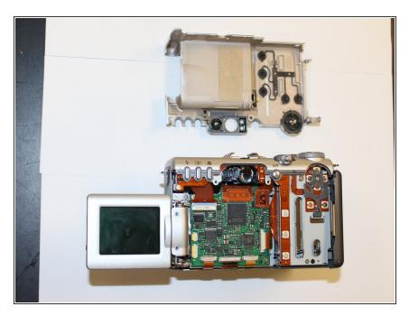
Once the screws are removed, remove the back panel. The panel should be able to be removed by hand.
