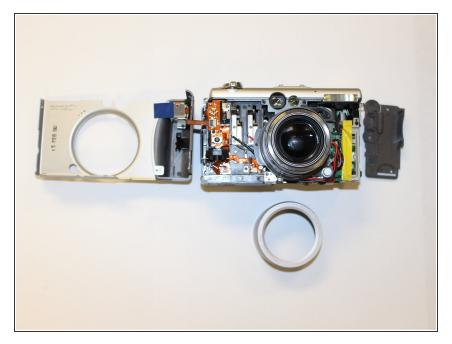
Next remove the front and right side panels (the left is attached to the front panel).
