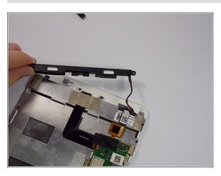
Lift out the speaker assembly form the plastic frame.
