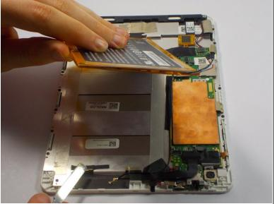
Un-stick the battery from the metal plate using the black nylon spudger.
