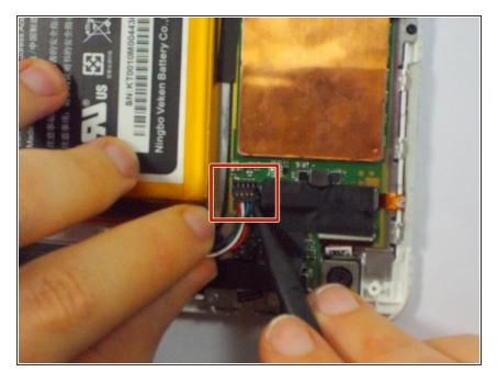
Remove the battery cable by lifting it up with the pointy end of the black nylon spudger.
