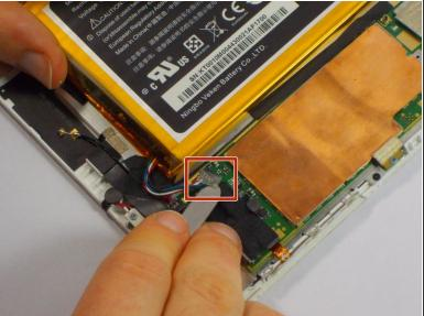
• Remove the small clear plastic cover on top of the battery cable with the nylon or metal spudger.
