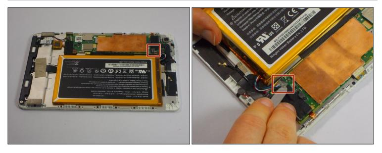
• Remove the small clear plastic cover on top of the battery cable with the nylon or metal spudger.
