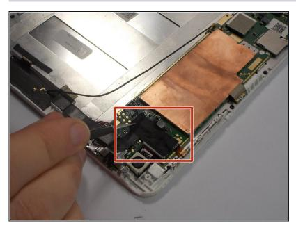
Peel off the piece of black tape covering the front facing camera ribbon cable connector.
