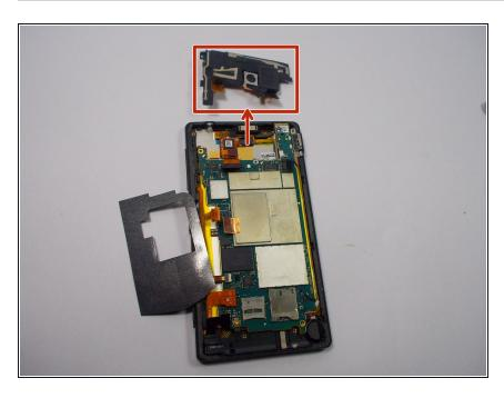
With all the connectors removed we can safely pry off the camera and all of its components using a plastic prying tool.
