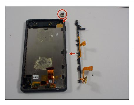
Next pry off the long plastic piece that goes around the perimeter of the left side of the phone. This part contains the volume and power button. The little component where the camera goes will need to be removed. Be careful when removing the front camera components because there is adhesive tape under it.
