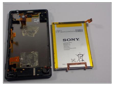
Take a small plastic prying tool and pry out the battery. The battery has adhesive tape that connects it to the phone which can make it difficult to pry out. Make sure to try prying from different angles of the battery.
