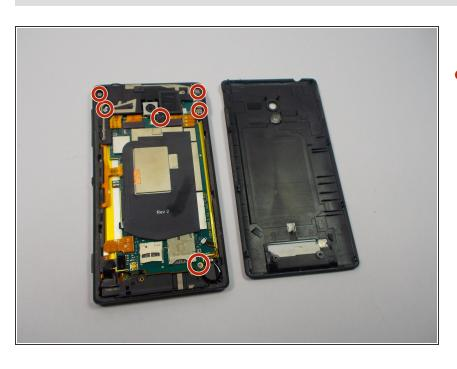
Remove the six screws from the phone using a JIS #00 screwdriver.
