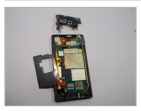
Remove the camera assembly using an opening tool or spudger.
