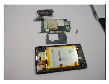
Remove the motherboard with an opening tool or spudger.
