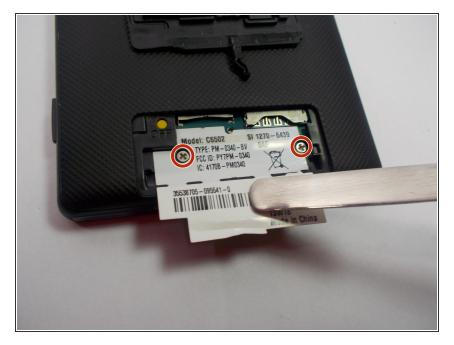
At the bottom of the phone will be a cover that flips open. A sticker will be under and when the sticker is peeled back, two screws will be revealed. Use a JIS J00 screw head to unscrew.
