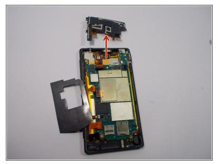
Once all the connectors have been disconnected. You will want to use a small prying tool to pry out the back camera and all its components from the phone.
