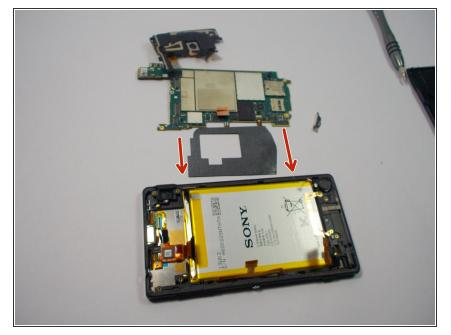
• Remove the electrical panel with a plastic opening tool.
