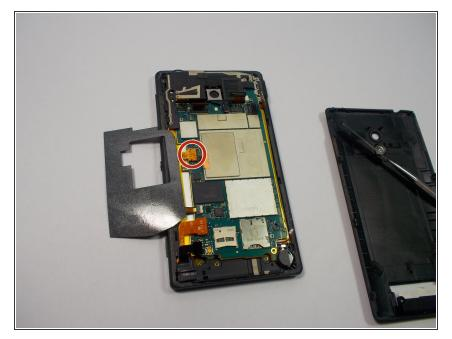
• The last connector is located under the black sticker. Peel back the black sticker and disconnect the last connector.
