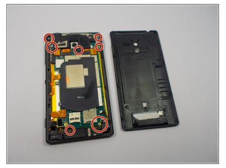
Once the two screws have been removed. Take the prying tool to pry off the back cover of the phone.
