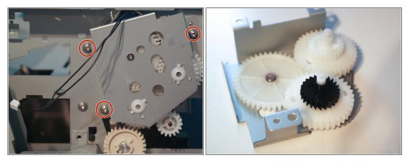
• Remove 3 screws holding the duplexer gears to the printer and remove the gears.
