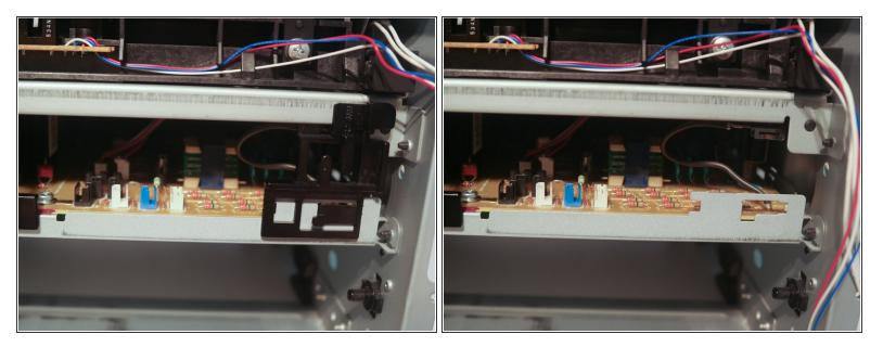
• Remove the cable guide from the chassis.
