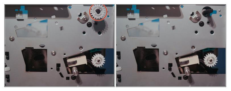
• Remove the fuser gear by pushing in on the tab with a metal spudger.
