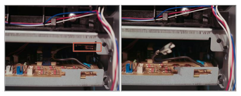
• Use needle nose pliers to disconnect the high voltage wire from the fuser.
