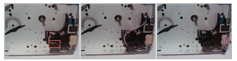
• Disconnect the cable to the tray connector and route it through the hole in the chassis.
