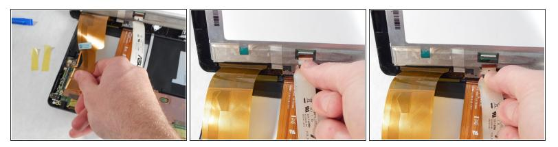
• With all three white levers pushed in, gently pull on each display cable until the cable disconnects.
