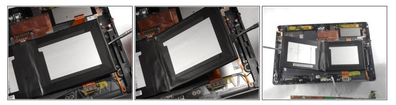
• Use the nylon or metal spudger to pry the battery from the back panel.
