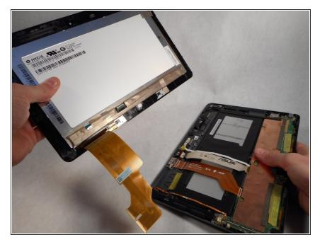
• Lift the screen upwards to remove.
