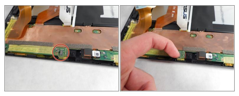
Before disconnecting the display cables, turn off the switch labeled DIP; this switch is used to deenergize the system.
