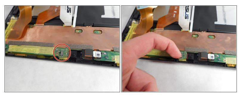
Before disconnecting the display cables, refer to the image to turn off the switch labeled DIP; this switch is used to de-energize the system.
