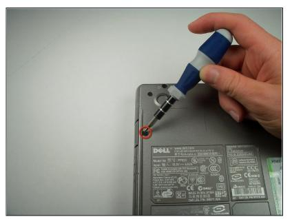
Locate and remove the screw that secures the CD-Rom Drive.
