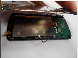
• Using a plastic opening tool or spudger lift the rear screen plate up and pull it off.
