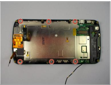
Use a T4 Torx Screwdriver to remove the (6) 1mm screws.
