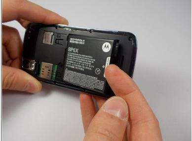
Remove the battery using the thumb tab.
