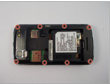
Using a T4 Torx driver, remove the eight 4 mm back panel screws.
