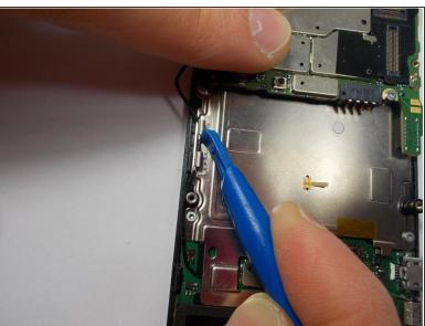
Disconnect the 2nd keyboard connector from the motherboard and remove it from its side holders.
