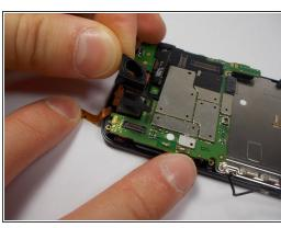
Remove the camera's rubber seal by pulling it off. It is not connected to anything.
